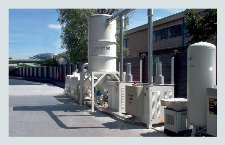
Pneumatic conveyors are an effective method to move dust and granules.
