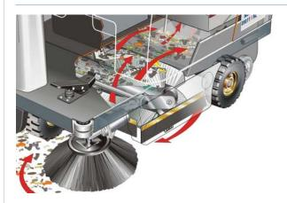
The container is placed BEHIND the main brush. The materials roll over the brush.
