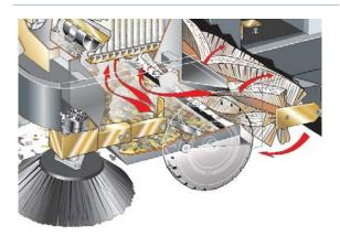
The container is placed IN FRONT OF the main brush. The materials that are loaded are pushed directly inside the container.
