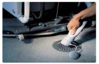
Splash-control hose prevents spillage while emptying tank.
