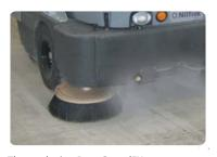
The exclusive DustGuard™ system effectively controls airborne dust by providing a fine mist of moisture to the front and side brushes.
