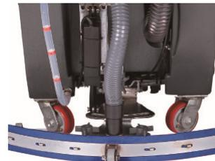
Electric actuator to adjust pressure
