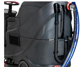
Built-in squeegee hanging system on recovery tank for easy machine transfer in narrow areas
